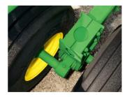
The wheel and tire configuration provide more flotation and even weight distribution across the entire machine
