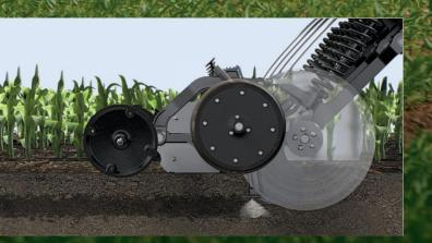
Applying on highly erodible land? The low-disturbance applicator leaves residue intact, so your customers can maintain conservation compliance.
